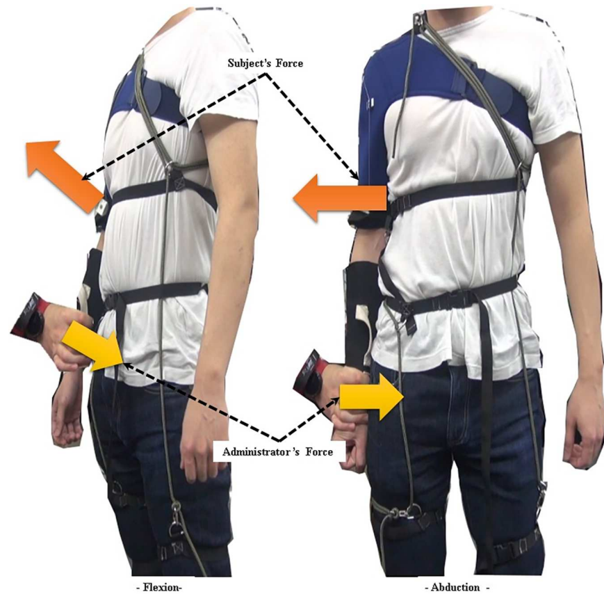
Fig 15. Experimental protocol. Measuring maximum voluntary contraction (MVC) in two directions, flexion and abduction.
