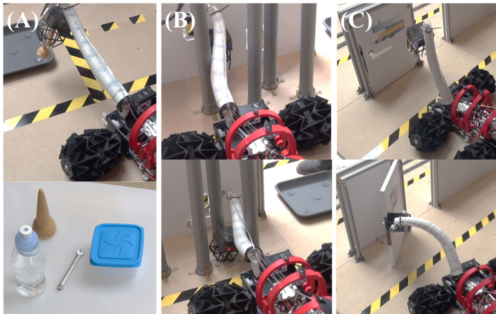
FIGURE 12 | Performance during the three manipulation scenario tasks. (A) Object pick and place task: SNUMAX picked up and placed all four objects with its PVSM and adaptive caging gripper. (B) Arm-positioning task: SNUMAX's PVSM reached all three target positions. (C) Door opening task: Lifting the PVSM while pulling the door allowed SNUMAX to manipulate the door knob and open the door.
