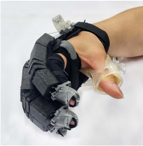
Fig. 1. Overall design of the proposed soft, cable-driven robotic glove with novel passive extensor mechanism.
