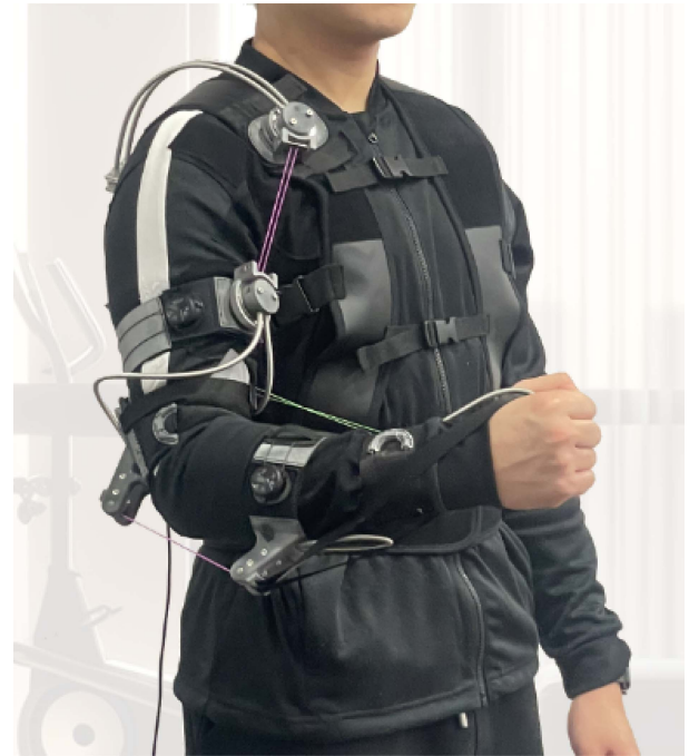
Fig. 1. Overall design of the cable-driven exosuit for bidirectional upper limb resistance exercises.
