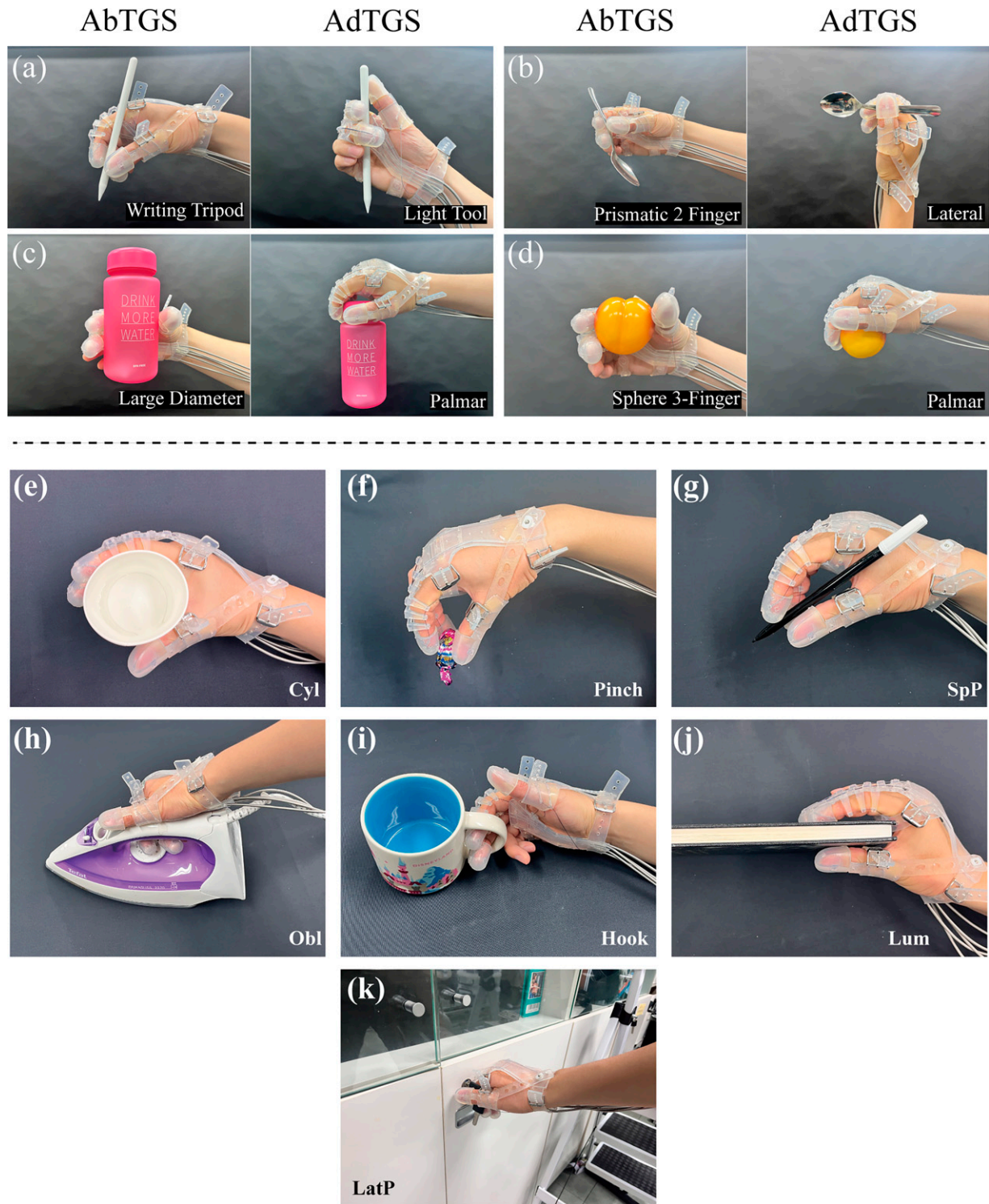
FIG. 10. Photographs demonstrating the subject grasping daily objects with EGP III. (a–d) Each grasp posture (in each legend) is classified according to the grasp taxonomy. 8 Grasping a pen, a spoon, a bottle, and a plum (mockup). The left column shows results with the AbTGS, and the right column shows results with the AdTGS. (e–k) The name of the grasp posture is referred from a previously reported categorization. 29 Grasping a paper cup with a cylindrical grasp (Cyl), a candy with a pinch grasp (Pinch), grasping a pen with special pinch (SpP), grasping an iron with an oblique palmar grasp (Obl), grasping a mug with a hook grasp (Hook), grasping a book with a lumbrical grasp (Lum), and grasping a key with a lateral pinch (LatP).
