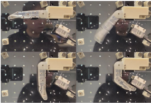
Fig. 3 Under-actuated PDVT finger free movement
